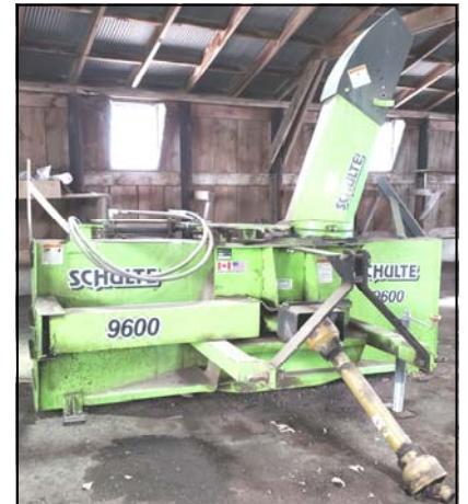
Schulte 9600 3 pt. snowblower w/ hyd. spout & 540PTO. Nice condition.
